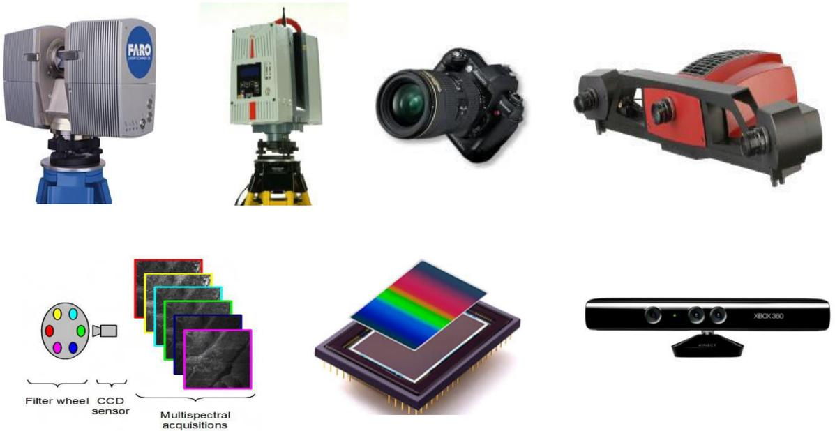
Figure 1: Example of sensors used for CH object digitalisation
