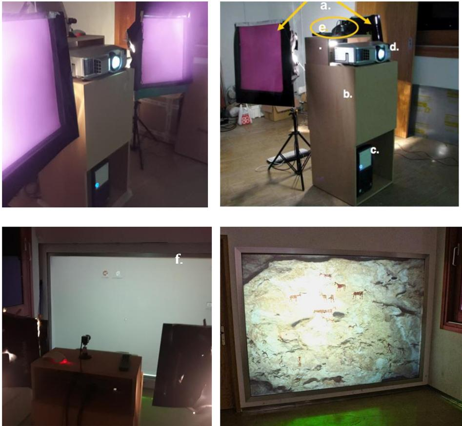
Figure 3. The main technological components of “We Hunters”. From left to right and top to bottom: infrared lights; overall view; back side of the screen; front side of the screen.
