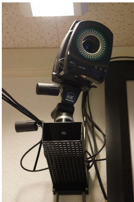
Figure 2: IR based cameras used to track suit markers
