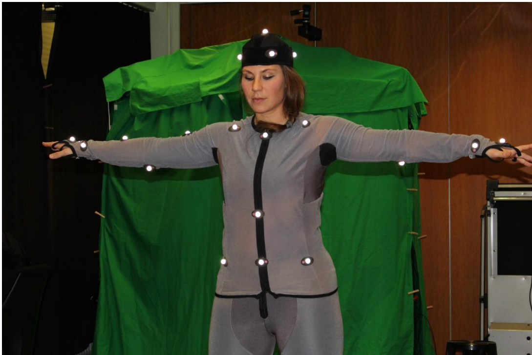
Figure 3: The pattern of markers placed on the body correspond to a standard, but can be modified.
