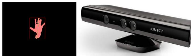
*Fig. 2: Tracked Hand. The position of the center of the hand is determined in real time by a Microsoft Kinect V1 that provide depth information*
